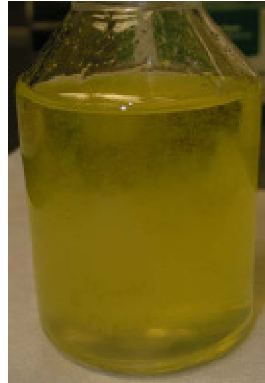
Cold Soak: ppt. above cloud point
