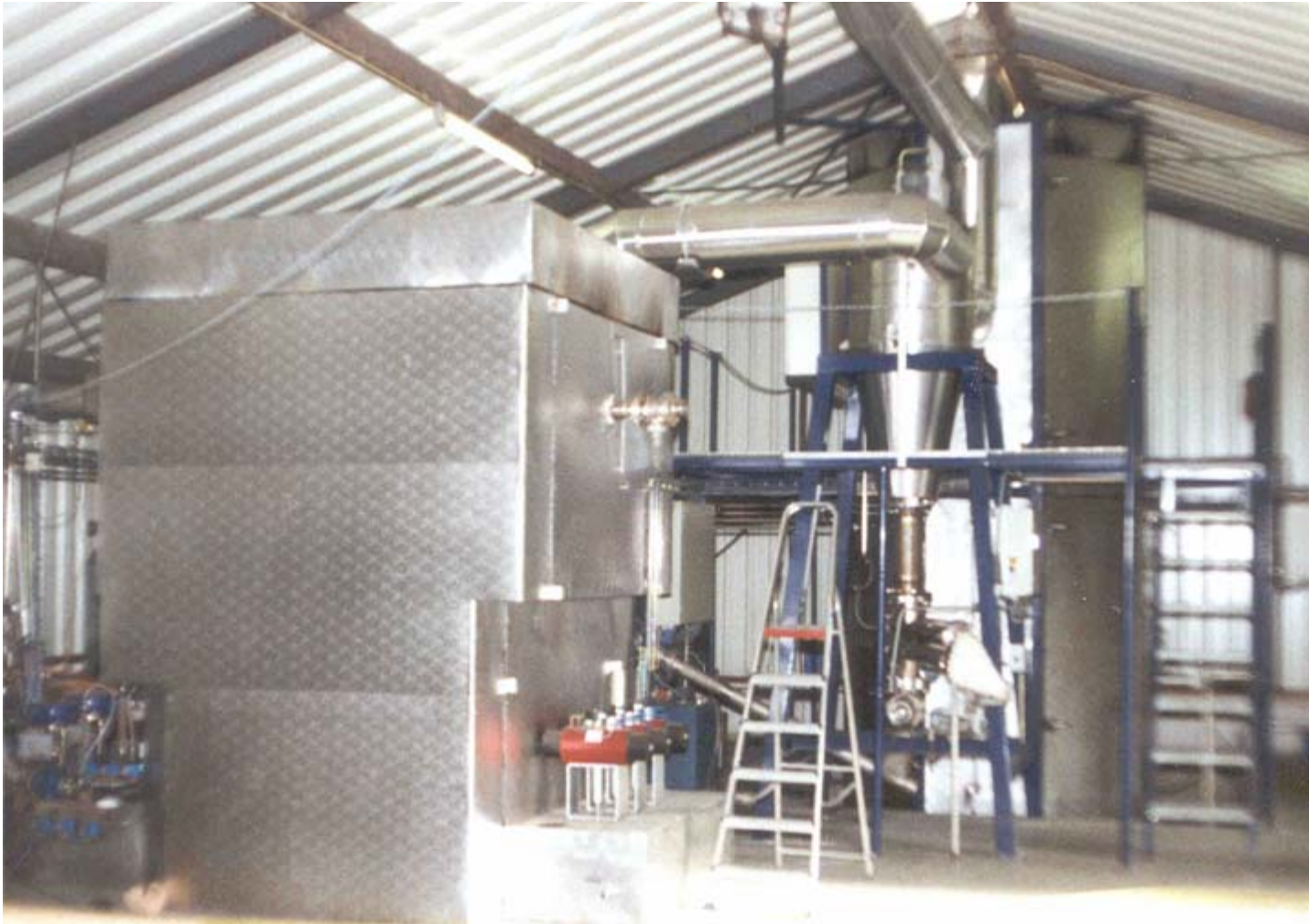
900 t/year chicken manure gasification plant (Bladel, NL)
