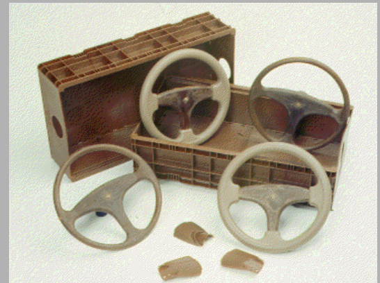
Injection moulded products from natural- fibre/plastic granules
