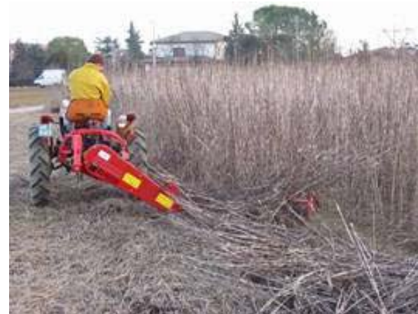
Gaspardo FBR 175 reciprocating a knife and teeth mower
