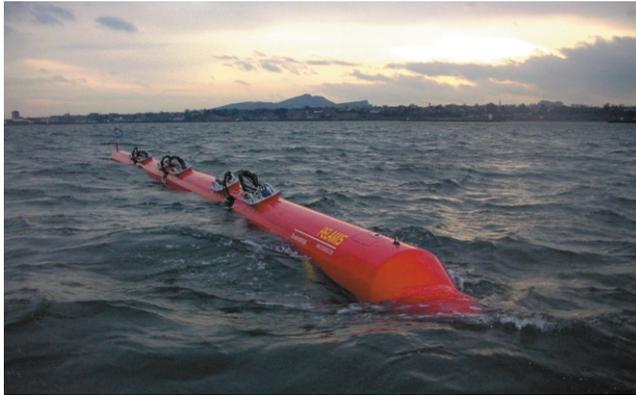
The **Pelamis**<sup>27,28</sup>, device is a semi-submerged articulated structure composed of cylindrical sections linked by hinged joints. The wave induced motion of these joints is resisted by hydraulic rams which pump high pressure oil through hydraulic motors via smoothing accumulators. A 130 m
