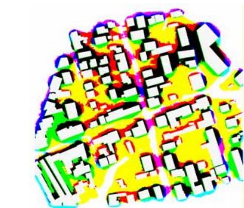
Wind shadowing contours of Thermi site, darker areas correspond to higher wind speeds
