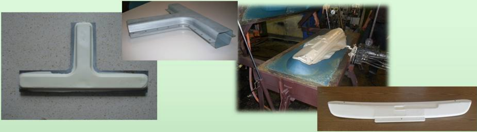
T-bone and spoiler for automotive by IWC, PEMU and CRF 25% renewable material
