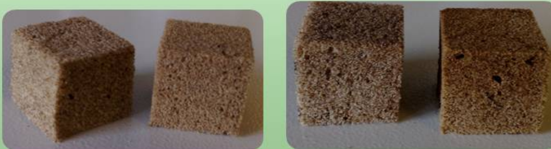
Soft PU foams by UNIPI with lignin content from 6% to 13% and total content of renewable material over 40%
