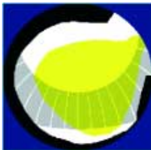
Figure 6.6: The multistereographic projection of the sky vault is split into three zones (black=sky directions obstructed on more than 80% of the site area, yellow=sky directions obstructed on less than 20% of the site area, white=criterion met). Finally, the sunpath diagram calculated for the latitude of the site is superimposed.
