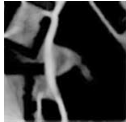
Figure 4.8: Wind Shadowing Map. Obtained from wind simulation snapshots of 12 different wind origins, this map shows the annual average frequency of wind flow. Darker areas correspond to areas with less wind.
