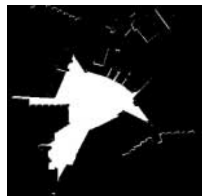
Figure 4.11: Viewshed Map. A mapping of the field of view from the middle of the site. White areas correspond to areas and surfaces within the person's potential line of sight (Matlab algorithm by Ratti [1]).
