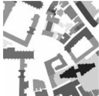
Figure 4.2: Digital Elevation Model (DEM). A greyscale 2D image with values ranging from 0 (black) to 255 (white), where black and white correspond to the highest and lowest heights of the area, respectively.
