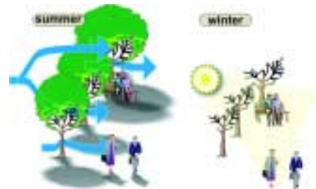
Figure 8.2: Deciduous trees offer shading in summer and if properly selected, can enhance air cooling by evapotranspiration. In winter they permit solar exposure of the site.
