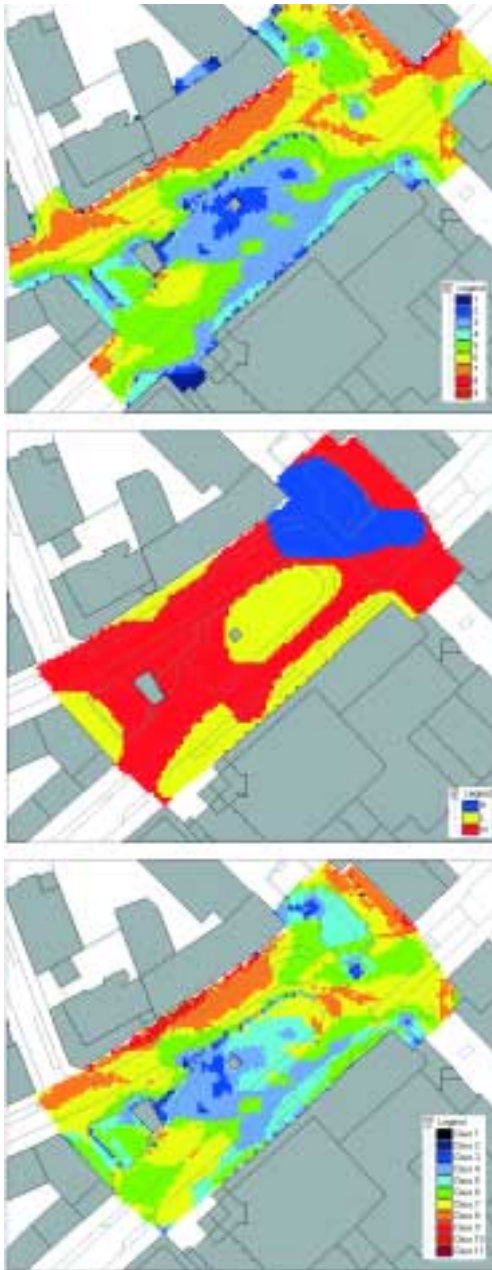
Figure 5.5: The thematic layers "radiation" and "wind" as well as the resulting "thermal comfort zoning" for Florentiner Platz.
