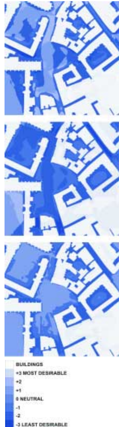
Figure 4.14: Desirability Map. (Top to Bottom: Summer, Winter and Annual Mapping) Seasonal and Annual desirability mapping based on the Diversity Profile (Figure 4.13) and a ranking of general preferences (Table 4.1). Darker areas indicate a lesser degree of desirability.
