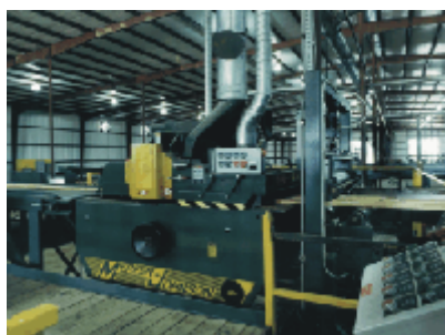
Figure 4.2. One of several saws and milling machines connected to a plant-wide industrial vacuum system
