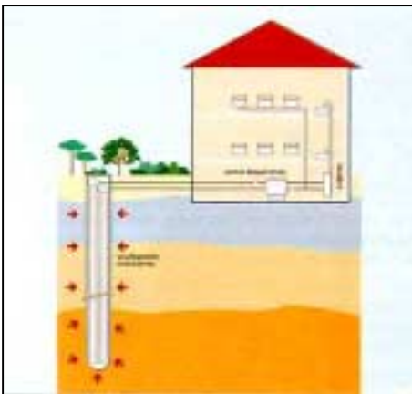
Geothermal system for house heating and cooling with water heat pump and geothermal heat exchanger
