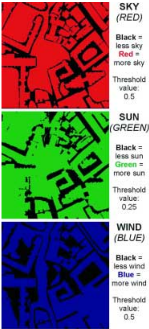
Figure 4.12: Sky, Sun, and Wind Threshold maps used as RGB channels for the Diversity Map (Figure 4.13).
