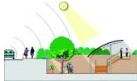
Figure 8.4: "Sunken" open spaces are an interesting solution to noise and wind protection. Tall shading devices can be easily used without interrupting the view beyond.
