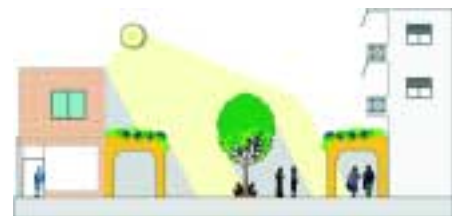
Figure 8.3: Galleries along a pedestrian zone can provide shading and protection from rain.
