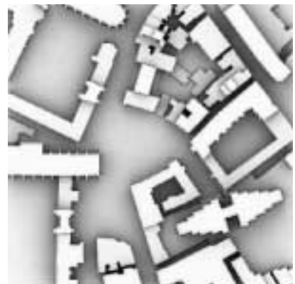
Figure 4.4: Sky View Factor Map. Lighter shades of grey correspond to higher sky view factors. (Matlab algorithm by Ratti [1]).
