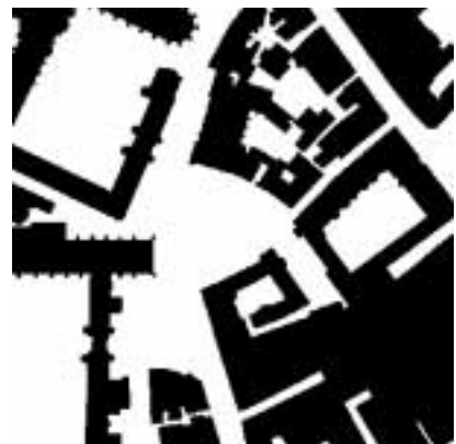
Figure 4.3: Figure Ground Map. A black and white image where black (0) corresponds to built-up area while white (1) corresponds to open space.
