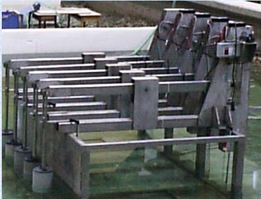
1:15 scale model of five converters in front of breakwater in the wide wave tank of NTUA
