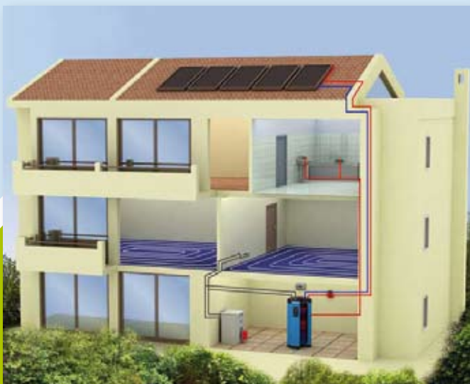
Layout illustration of a typical solar thermal system which covers building's floor heating and SHW needs.
