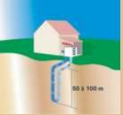
Typical piping material is HDPE (High Density Polyethylene), which has a life expectation of at least 50 years in this application, and typical external pipe diameters are 32 or 40 mm. Depending on the design operation temperature range, the pipe may be filled with water or a mixture of water and antifreeze.
