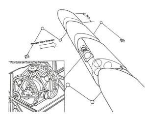
The concept of the **Salter Duck**<sup>31</sup> was introduced in 1974 by S. Salter<sup>32</sup>. An important feature of this device is the capability of converting both the kinetic and potential energies of the wave, achieving thus very high absorption efficiencies (theoretically over 90%). The system has undergone considerable development since 1983 and it was
