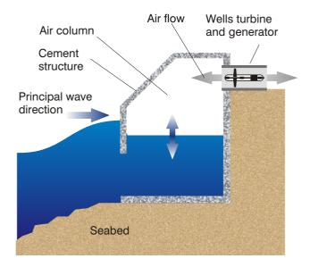
One major class of shoreline devices is the oscillating water column (OWC). It consists of a partially submerged, hollow structure, which is open to the seabed below the waterline. The heave motion of the sea surface alternatively pressurizes and depressurizes the air inside the structure generating a reci-pro-
