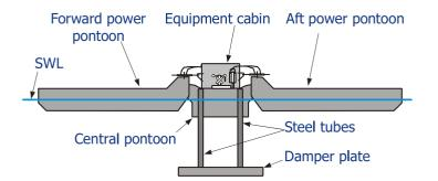
The McCabe Wave Pump<sup>23,24</sup>, consists of three rectangular steel pontoons, which are hinged together across their beam. The bow of the
