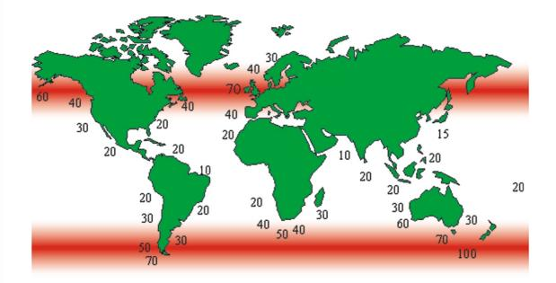
Figure 1: Global wave power distribution in kW/m of crest length
