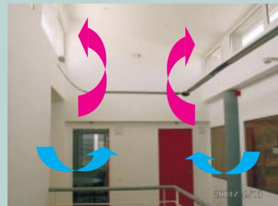
The solar atrium is used as a passive cooling system, for direct natural lighting and solar radiation
