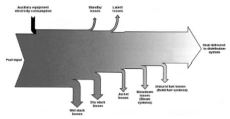
Figure 4.14. Energy flows in a boiler-burner central system
