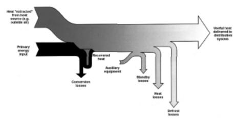
Figure 4.16. Energy flows in a central heat pump system (Heating operation)
