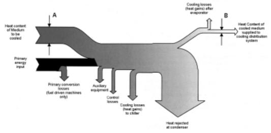
Figure 4.15. Energy flows in central cooling plant (A-B = Net cooling output delivered to the distribution system)
