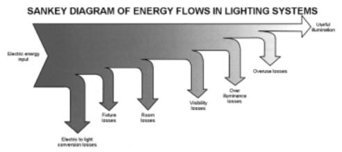
Figure 4.19. Energy flows in an artificial lighting installation
