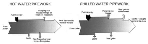
Figure 4.17. Energy flows in water distribution piping systems
