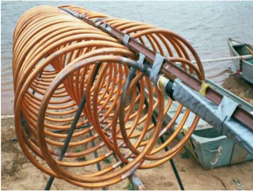
Fig. 2. Copper Lake/Pond Loop was constructed and installed on the campus of Oklahoma State University. The heat exchanger is constructed from 25 mm diameter copper pipe with a total length of copper pipe of 91 meters. Rated capacity is 1.5 kW.
