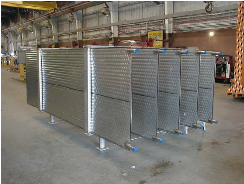
Fig. 3. 12-kW pre assembled stainless steel plate pond loop. Photograph supplied by AWEB Supply – Baton Rouge, Louisiana
