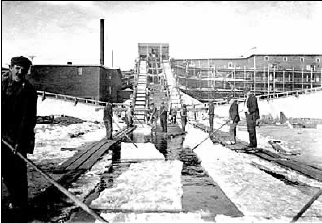
Fig. 2. Ice is being harvested from the frozen lake surface and stored to provide refrigeration and air conditioning the following summer. Photo from www.fauerbachbrewery.com/iceharvesting.htm .
