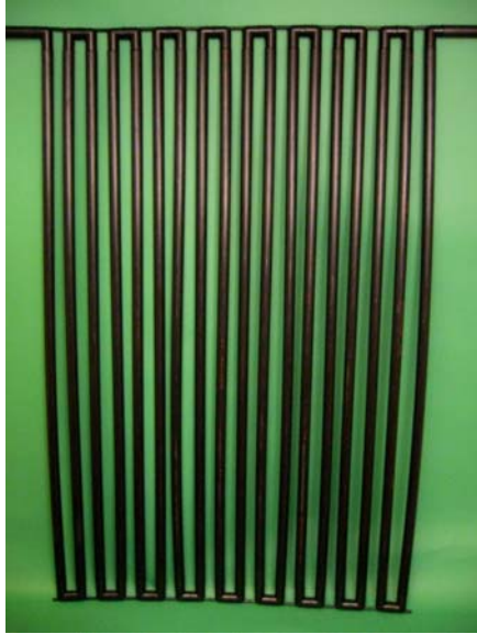
Fig. 6. Compact collector module and a top U-bend
