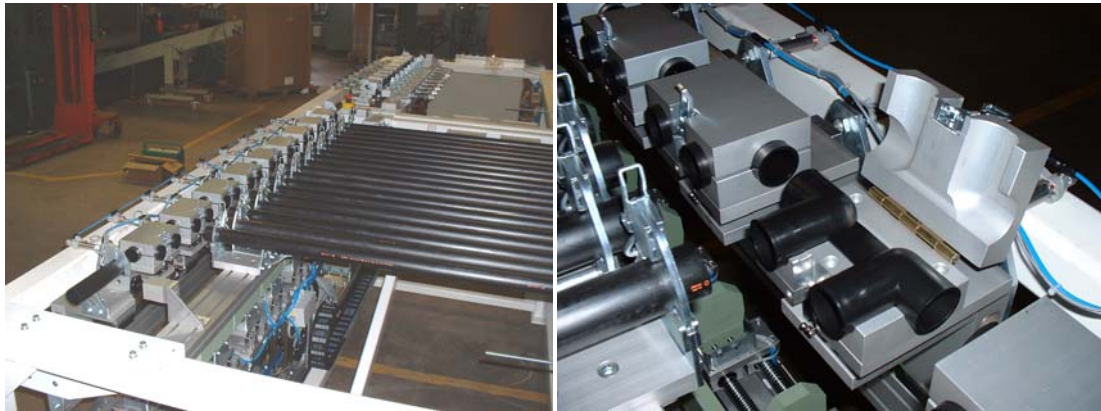
Fig. 7. Mirror welding machine for compact collectors
