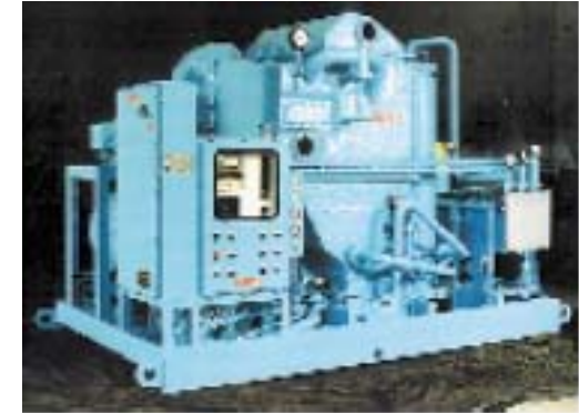
A mechanical vapor compression unit
