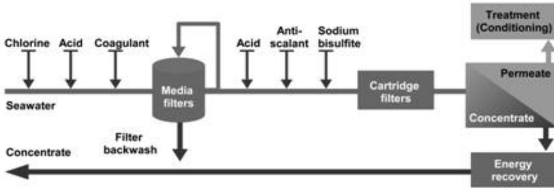
Flow-chart of an SWRO system showing the conventional pretreatment and chemical addition steps
