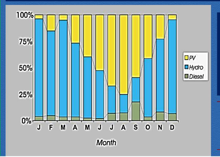
The Diesel Generators are used for peak demands and backup, with usually less than 800 operating hours p. a.
