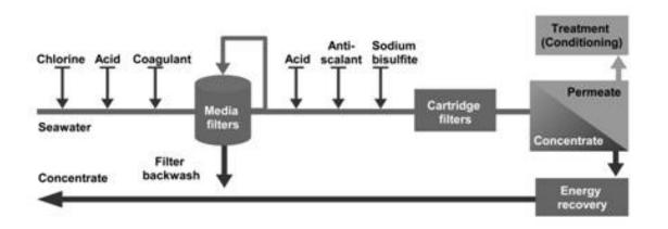
Flow-chart of an SWRO system showing the conventional pretreatment and chemical addition steps
