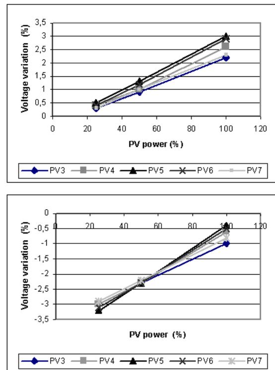
Figure 6: Voltage variation as a function of photovoltaic power injection, for the light load condition (top) and heavy load condition (bottom).
