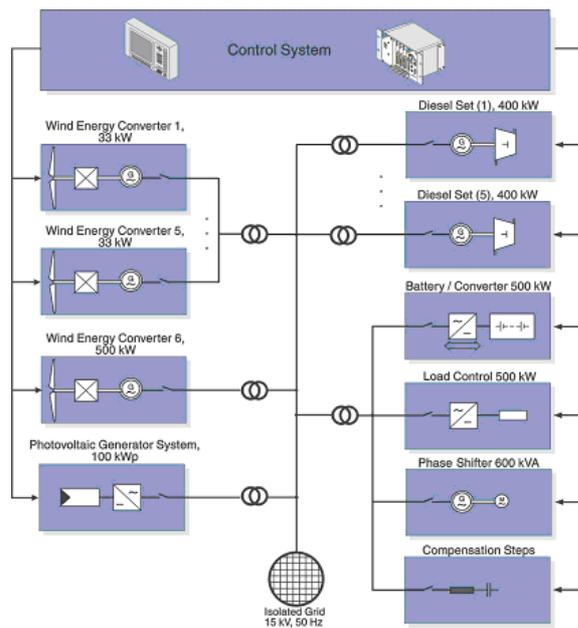
Figure 1: Kythnos power system block diagram.
