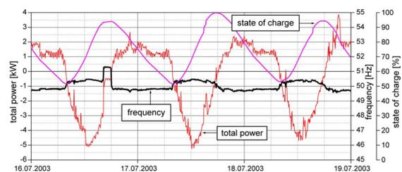
Figure 3: System control in a micro-grid by means of varying system frequency: In case of power surplus the battery is charged and the positive energy balance is indicated by a higher system frequency ( $\approx 50.5\text{Hz}$ ). When the battery is nearly completely charged the system frequency is raised additionally by the energy management system ( $\approx 51.3\text{Hz}$ ). This is recognised by the PV inverter and the PV power is limited in order to avoid overcharging of the battery.
