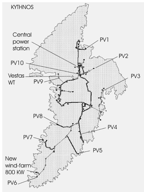
Figure 5: Kythnos medium voltage grid and the power sources locations.
