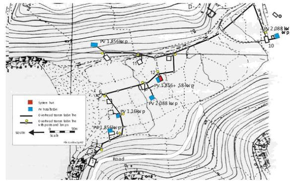
Figure 2: The house numbers, size and location of the PV arrays at the settlement of Gaidouromantra in Kythnos.
