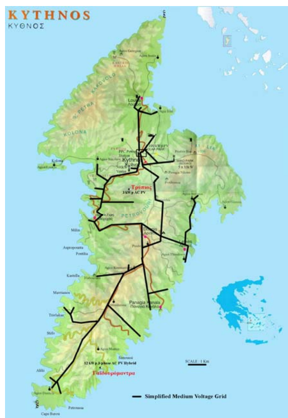
Fig. 5. A simplified version of the medium voltage network supplying the island of Kythnos.
