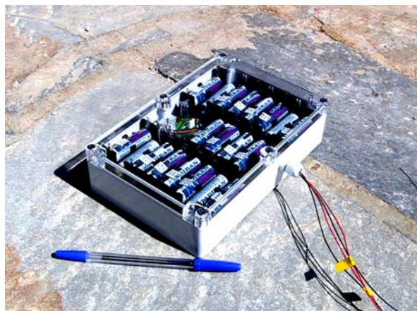
Figure 2. Final high-level BMS hardware
