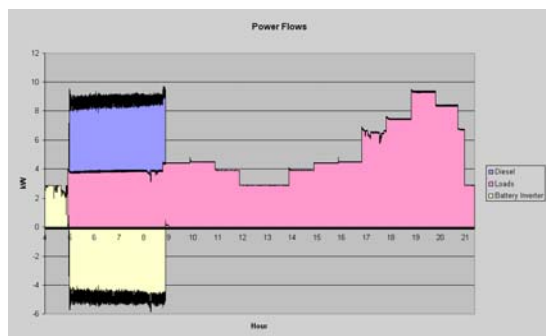
Figure 10: Power flows of the diesel generator, the battery inverter and the load demand.
