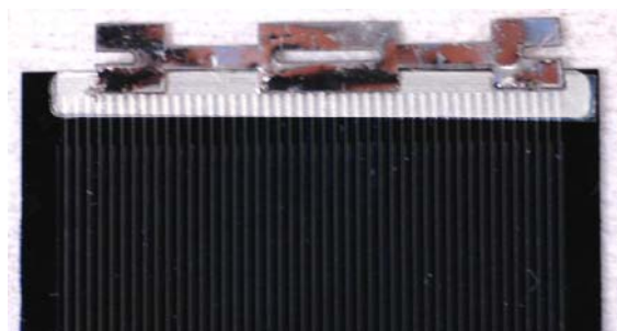
Figure 4: Metallised rear side of the bifacial cell fabricated within the REFLECTS project. The busbar connects the obliquely evaporated contact fingers. The connector bone is soldered to the unstructured part of the evaporated busbar.
