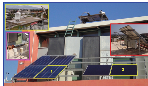
Figure 1: CRES long-term PV module testing field, weather station and measuring system equipment.
