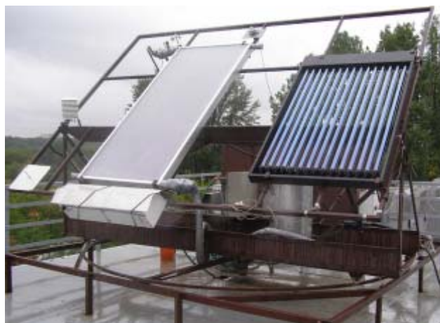
Figure 40: Station in Institute for Buildings Mechanization and Electrification of Agriculture in Warsaw performing outdoor tests of solar collectors
