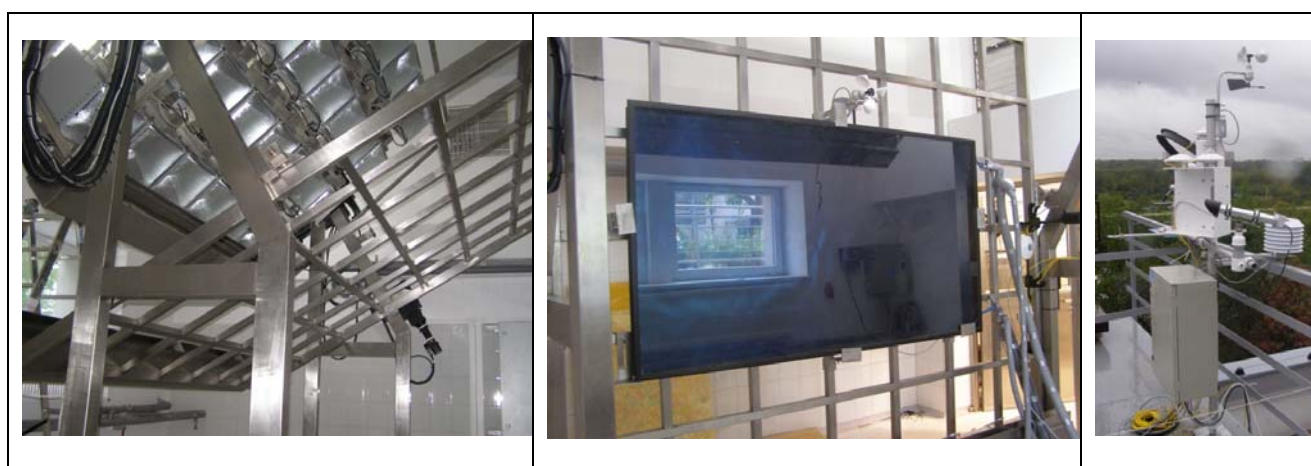
Figure 41: Station in Institute for Fuels and Renewable Energy in Warsaw performing indoor tests of solar collectors accordingly EN standards.
