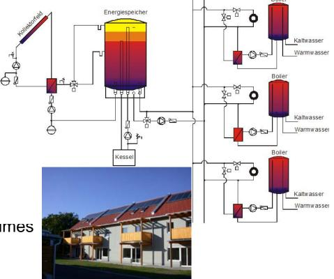
Advantage: Low return temperatures from the beginning of the boiler load
