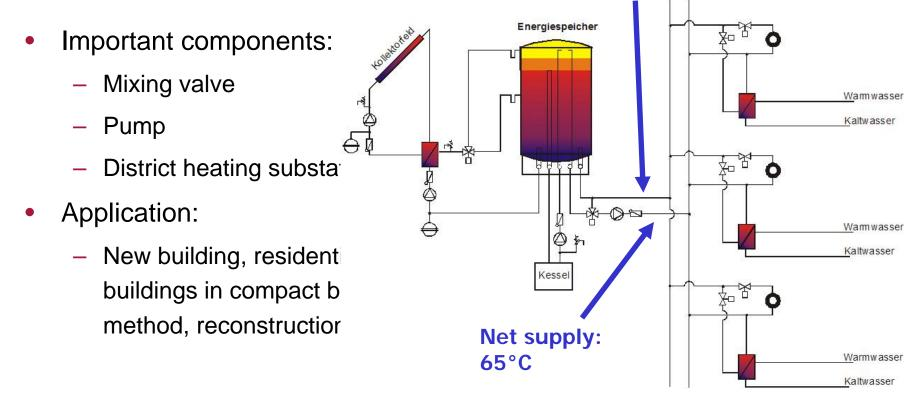
Advantage: The hole year low return temperatures of approximately 30°C → few distribution net losses
