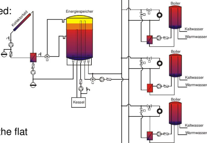
**Important:** The distribution net is used 22h to 23h for the heat supply and just 1h to load the boiler
