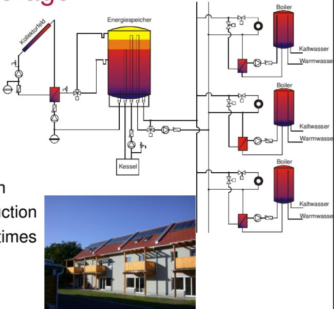
**Advantage: Low return temperatures from the beginning of the boiler load**
