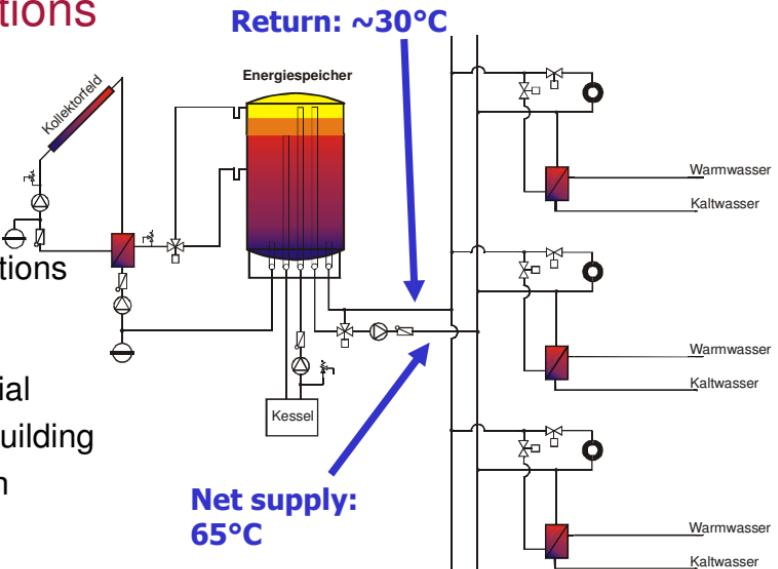
**Advantage: The hole year low return temperatures of approximately 30°C → few distribution net losses**
